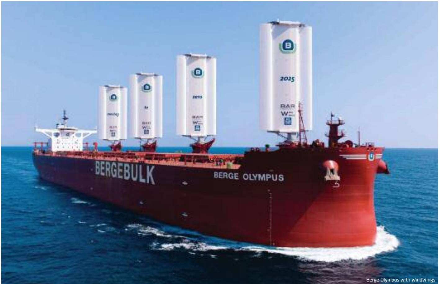
Berge Olympus with WindWings
