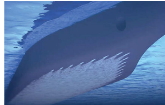
The Silverstream® system helps save 5-10% net fuel and emissions Source: Silverstream
