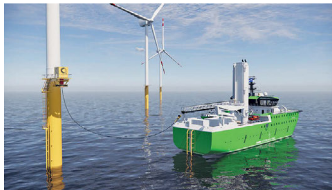
The CTV can either charge at a turbine or at one of Damen's CSOVs outfitted with a charger
